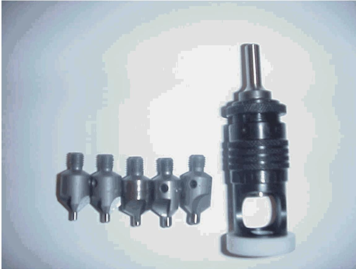
Dimpling is usually performed on homebuilts with the two disks mentioned earlier fitted into a hand pop rivet gun. The nail that runs through the disks is inserted into the gun like a rivet mandrel.
