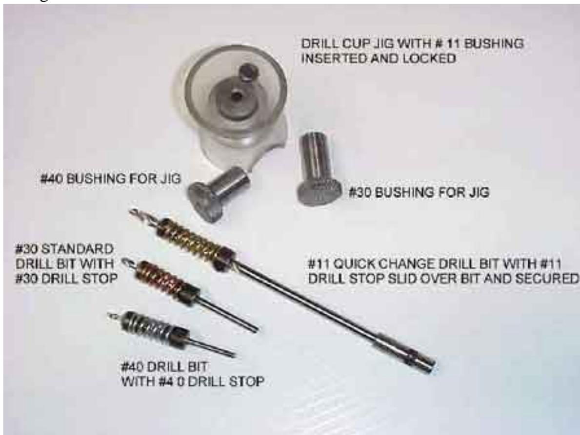
Drills, drill bits and holes. An aircraft is basically thousands of rivets and bolts flying in close formation. These squeeze various parts together, inserted through holes, many of which the builder has to drill. The industry calls these rivets, bolts, screws etc. “fasteners”.
